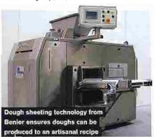
mating this process is that the dough used to make artisanal products is much more fluid than the dough used in standard breads. "These doughs will not go through mainstream dividers and moulders," Marsh says.
