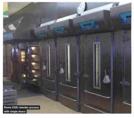
retarding and proving systems to cope with the production requirements of anything from a few trays upwards. Its GVA macbine has five programme sections: fast-cooling, proofing interruption, proofing retardation, proofing and the support phase. It can operate between -25°C and 45°C and with humidity levels between 68% and 98%.
